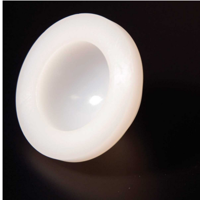
Figure 23: Example of a UHMWPE bushing, used in Snack Sack at the flap's pivot to provide a low-friction, wear-resistant bearing surface that increases the flap's opening angle.
