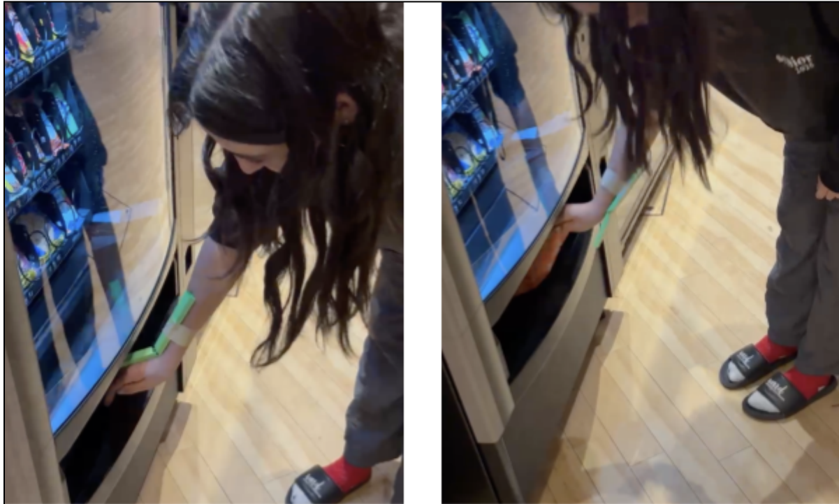
Figure 28: Testing for the wrist bending needed for retrieving products from an existing, normal functioning vending machine on Chestnut 27th floor. The left image depicts measuring wrist extension. The right image depicts measuring wrist flexion.
