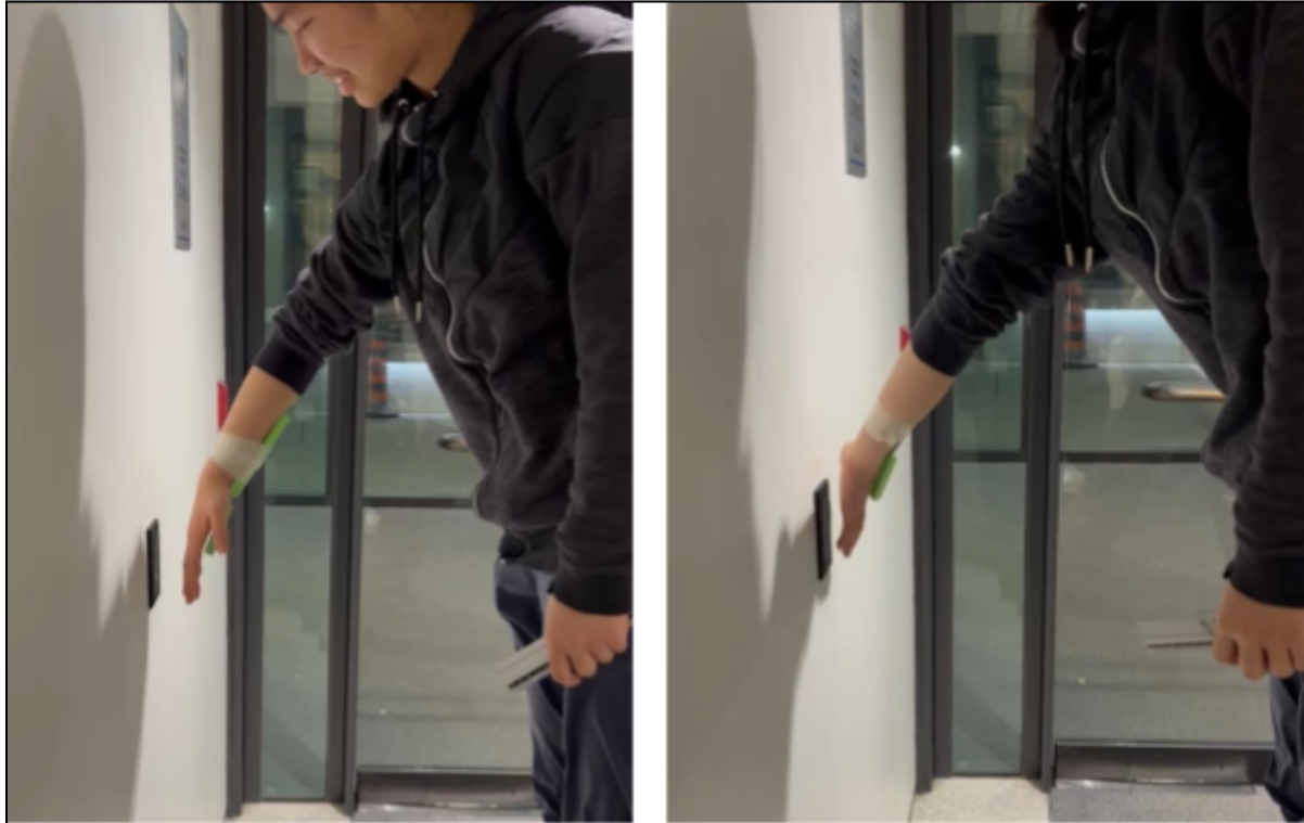
Figure 29: Testing wrist bending required to trigger a sensor near the Myhal first-floor entrance. Testers stood on a chair to replicate the intended user activation height. The left image depicts measuring wrist flexion. The right image depicts measuring wrist extension.
