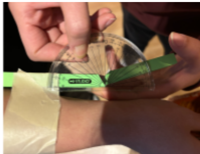
Figure [5.2]: Measuring the wrist flexion by attaching the device to the back of the wrist.
