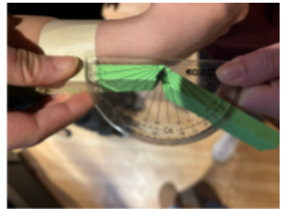
Figure [5.3]: Measuring the wrist extension by attaching the device to the front of the wrist.
