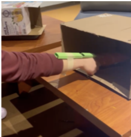
Figure [6]: Testing for the wrist bending needed for retrieving products from an opening with no obstruction. The left image depicts measuring wrist extension. The right image depicts measuring wrist flexion.
