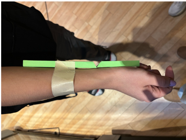
Figure 7: A wrist flexion and extension measuring device setup used for the wrist ergonomics proxy tests.
